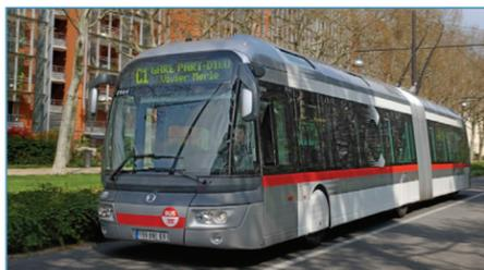
Features of a **bus rapid transit (BRT)** system include high-tech vehicles, dedicated busways and bus lanes, attractive and easily recognizable stations and stops, pay-before-boarding fare collection to avoid delays, and electronic signs that let riders know when the next bus will arrive.
